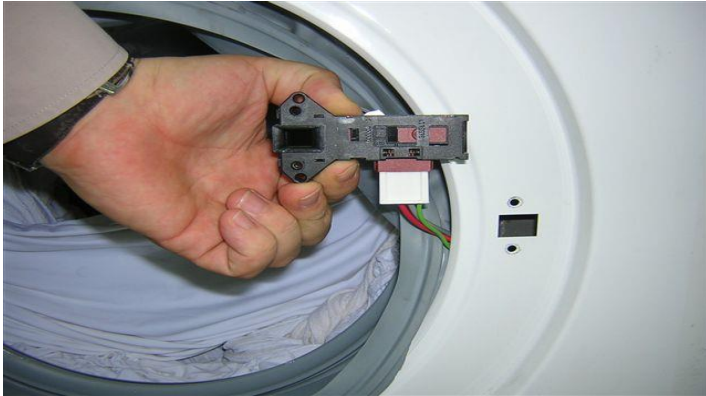
Picture 5.29 Disassembly/assembly of safety switch
