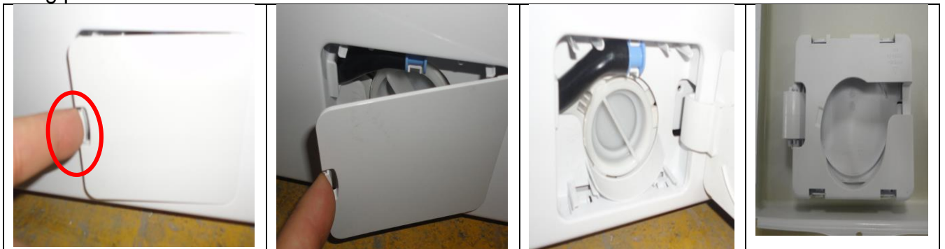
Picture 5.17 Pump cover Disassembly/Assembly
