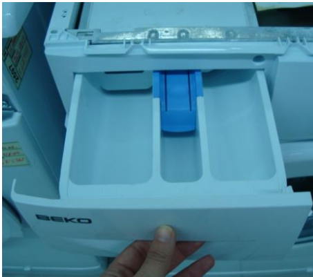
Picture 5.5 Disassembly/Assembly of Detergent Dispenser
