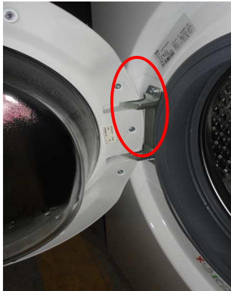
Picture 5.18 Front door disassembly /assembly
