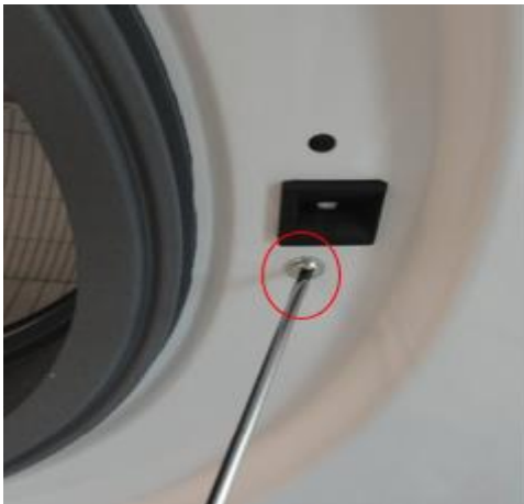
Picture 5.21 Front Wall Disassembly / Assembly
