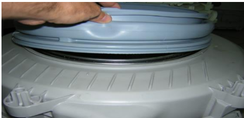
Picture 5.34 Disassembly/Assembly of Drum Bellows
