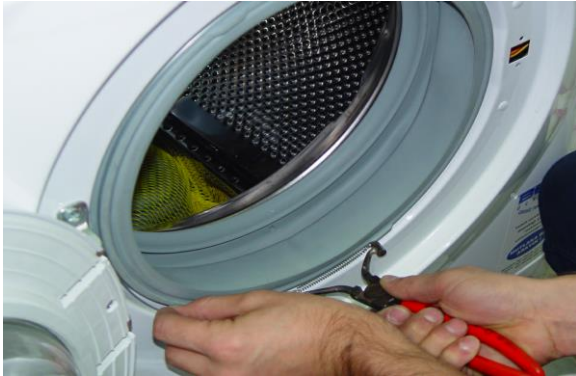
Picture 5.20 Front Wall Disassembly / Assembly
