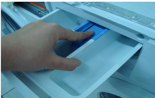
Picture 5.6 Disassembly/Assembly of Detergent Dispenser
