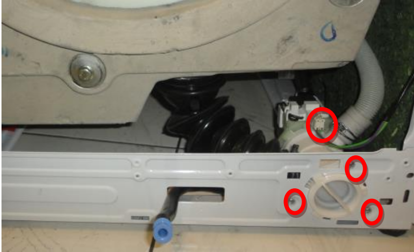
Picture 5.31 Drain pump Attachment/Detachment
