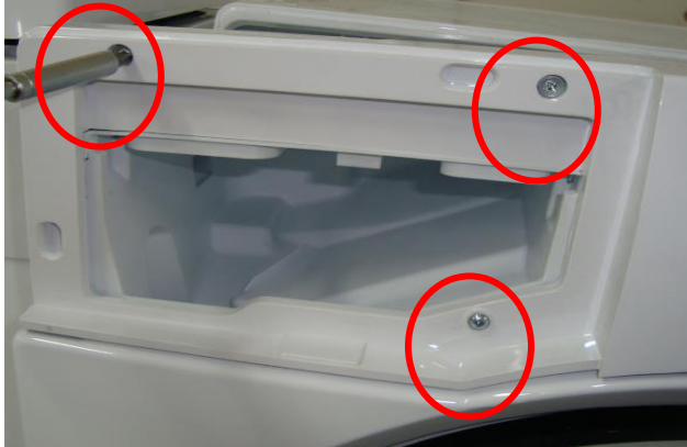
Picture 5.10 Panel Disassembly/Assembly
