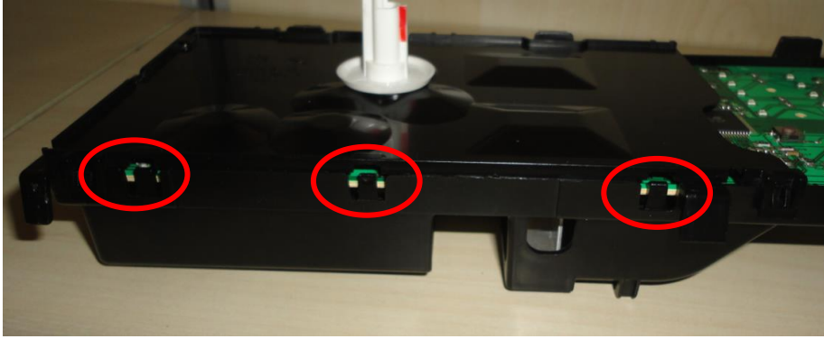
Picture 5.14 Control card Disassembly/Assembly
