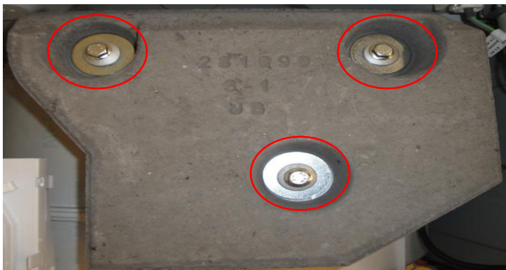
Picture 5.38 Disassembly/assembly of upper counterweight
