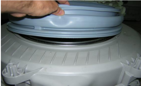
Picture 5.33 Disassembly/Assembly of Drum Bellows
