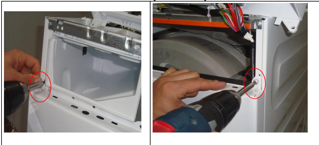
Picture 5.22 Front Wall Disassembly / Assembly
