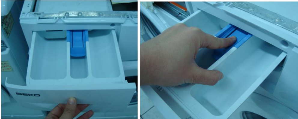
Picture 5.7 Panel Disassembly/Assembly
