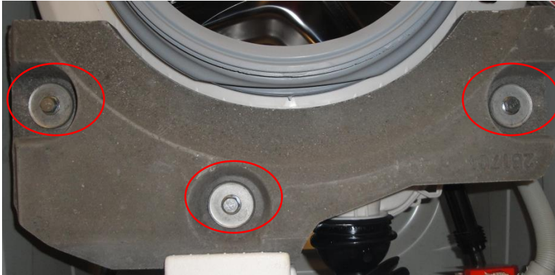
Picture 5.39 Disassembly/assembly of lower counterweight
