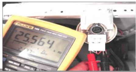
PICTURE E2-5: Water level sensor is being controlled
