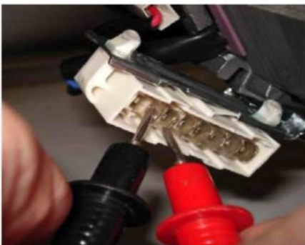
PICTURE E11-4: Motor coil resistance is being measured over 8-pin motor
