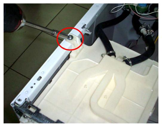
Tabs locking the panel on to the support bracket will be removed to release the panel from the support bracket.
