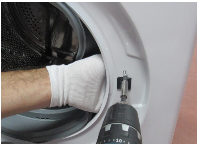
Tighten the door lock screw
