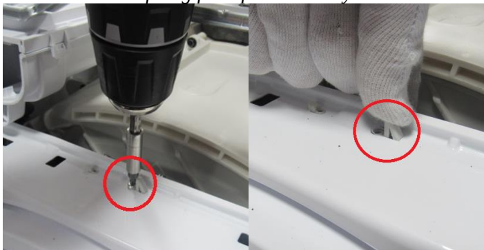
Remove the screw fixing twinjet elbow.
