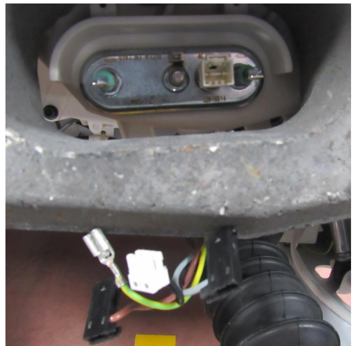
Remove the heater sockets
