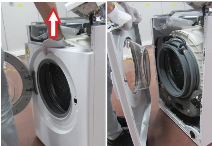
Pull up and remove the front panel.
