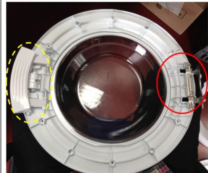
2.7. Remove the plastic parts as shown in the photo above.
