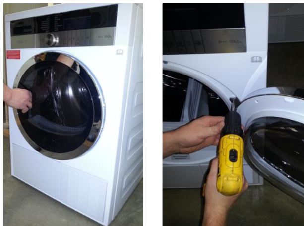
Figure 13.18. Unscrewing the door group
