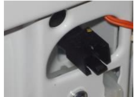
Figure 8.3. NTC located after the door filter in air suction channel
