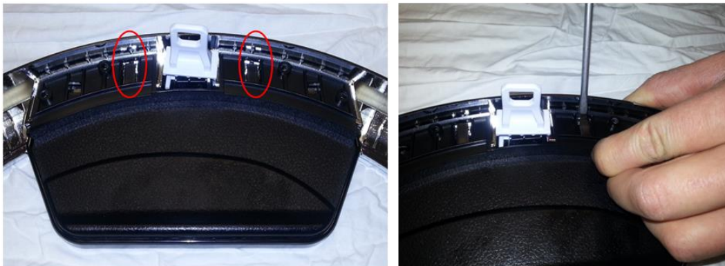
Figure 13.26. Removing the snap fits
