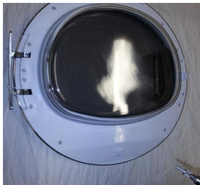
Figure 13.30. Screwing the door group
