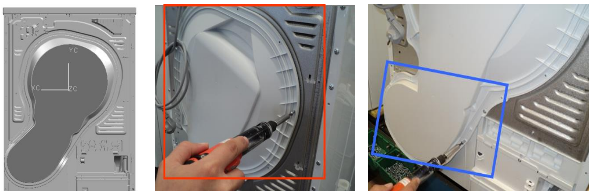
Figure 13.7. Connection points between the plastic cover - rear panel and plastic chassis
