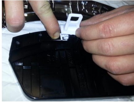
Figure 13.28. Removing the lock hook
