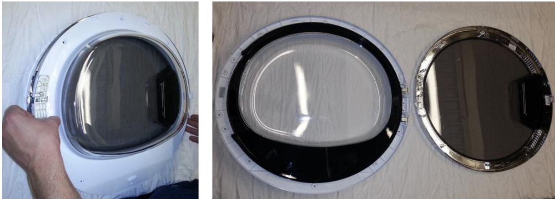
Figure 13.20. Removing the rear plastic door group
