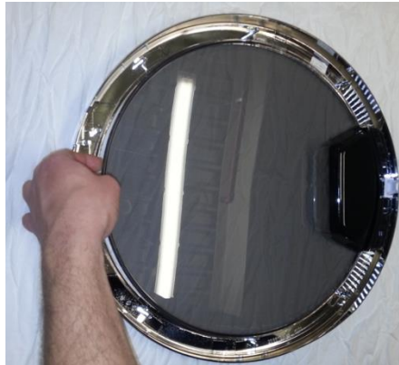
Figure 13.25. Removing the protective door
