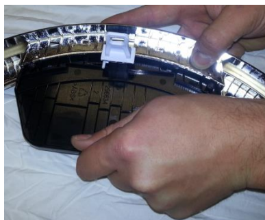
Figure 13.27. Removing the inner handle
