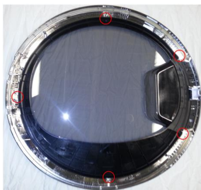
Figure 13.24. Fixing Points for the inner inlay
