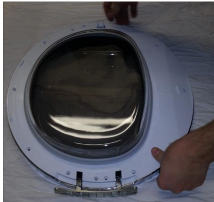
Figure 13.29. Assembling the door group
