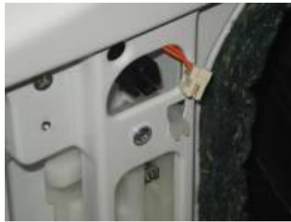
Figure 8.3. NTC located after the door filter in air suction channel
