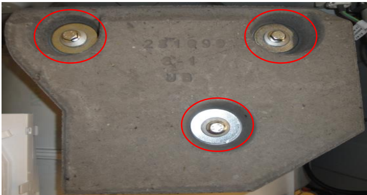
Picture 12.44 Disassembly/assembly of upper counterweight
