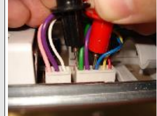
PICTURE E8-3: AC voltage is being measured over valve connectors
