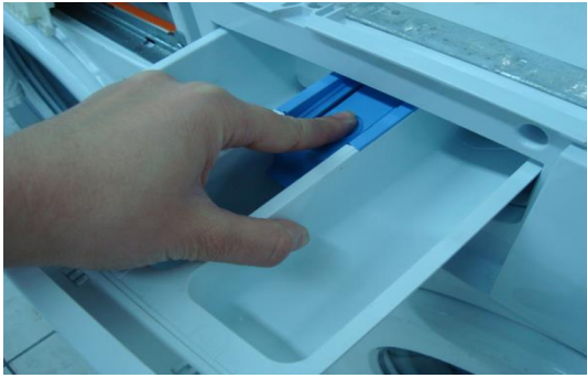
Picture 12.23 Disassembly/Assembly of Detergent Dispenser
