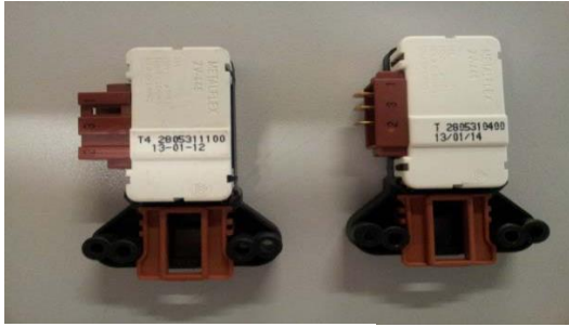
Picture 8.2 Safety switch
