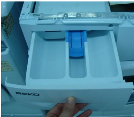
Picture 12.22 Disassembly/Assembly of Detergent Dispenser
