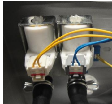
PICTURE E4-1: Water intake valves
