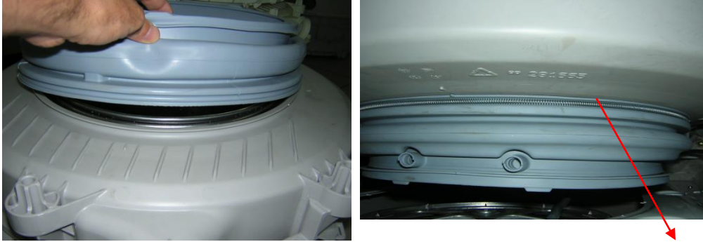
Picture 12.39 Disassembly/Assembly of Drum Bellows
