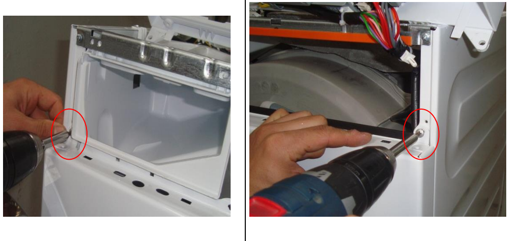
Picture 12.20 Front Wall Disassembly / Assembly
