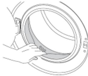
Figure 5.6 Cleaning the bellows
