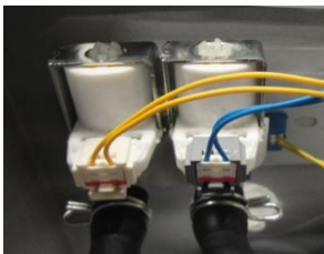
PICTURE E8-1: AC voltage is being measured over valve connectors
