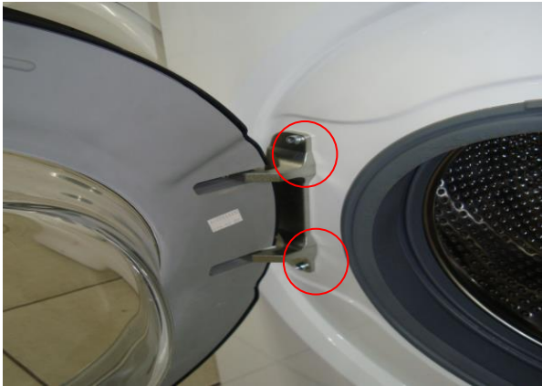
Picture 12.7 Front door Disassembly /Assembly
