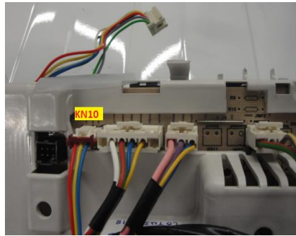
Picture E13-1: KN10 connector connection on the card
