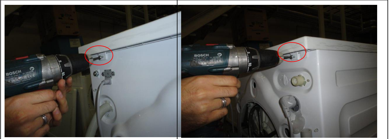
Picture 12.3 Upper table Disassembly/Assembly
