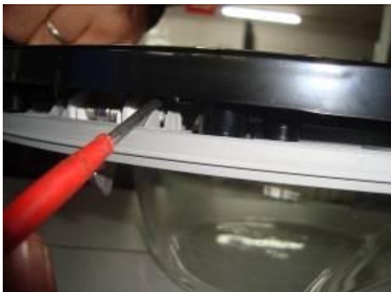
Picture 12.11 Assembly/Disassembly of Handle Cover
