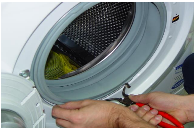
Picture 12.18 Front Wall Disassembly / Assembly
