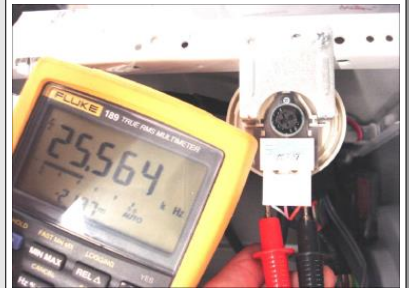
PICTURE E2-5: Water level sensor is being checked
