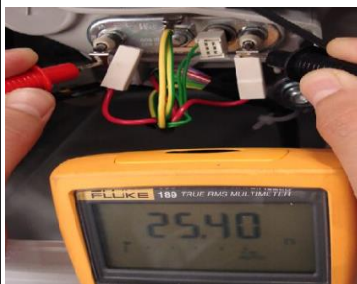
PICTURE E2-4: One of the cables on the heater is removed (left) and heater resistance is measured.
