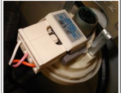
PICTURE E7-1: The socket on the level sensor must be fitted.
