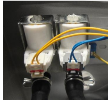
PICTURE E4-1: Water intake valves
