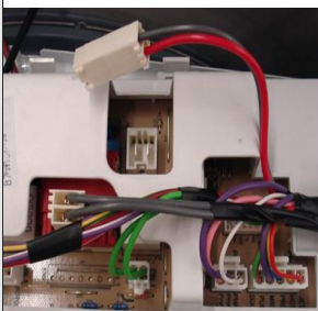
PICTURE E2-1: Heater socket on the KN5 card is removed.
