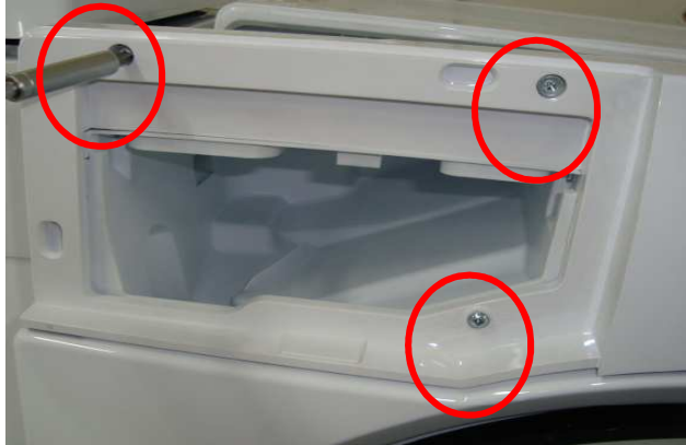
Picture 11.10 Panel Disassembly/Assembly
