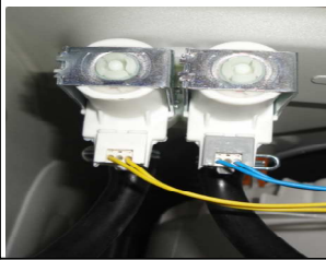
PICTURE E8-1: AC voltage is being measured over valve connectors
