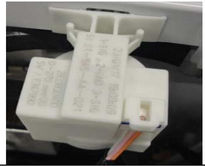
PICTURE E7-1: The socket on the level sensor must be fitted.
