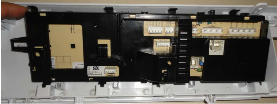
Picture 11.14 Control card Disassembly/Assembly
