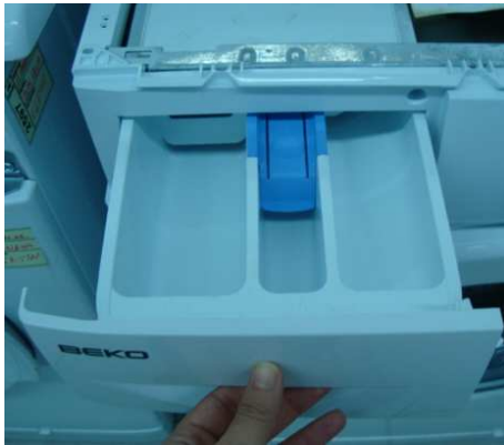
Picture 11.5 Disassembly/Assembly of Detergent Dispenser
