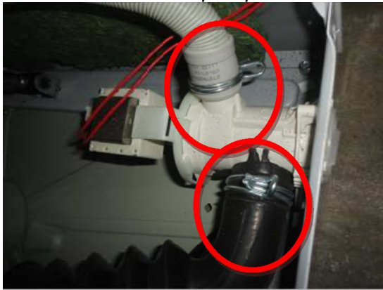
Picture 11.33 Drain pump Attachment/Detachment
