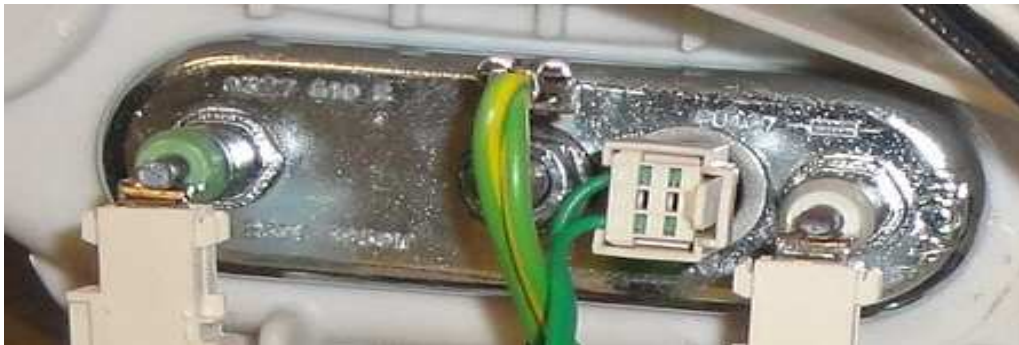
Picture 11.32 Disassembly/assembly of Heater
