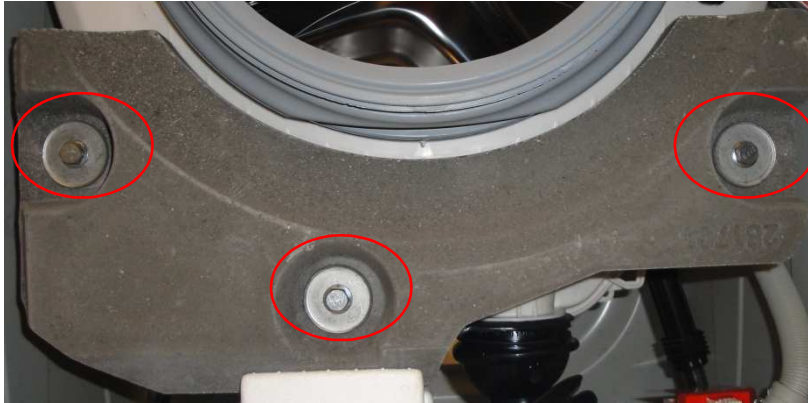
Picture 11.41 Disassembly/assembly of lower counterweight
