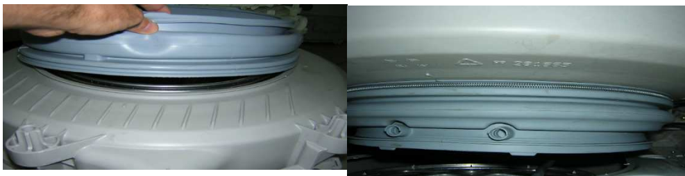
Picture 11.36 Disassembly/Assembly of Drum Bellows
