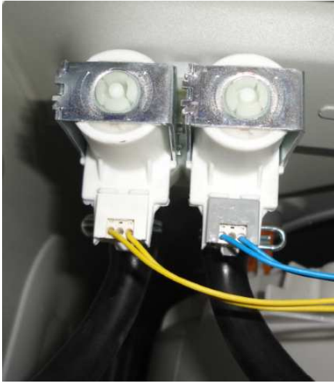
Picture 7.5 Water inlet valve
