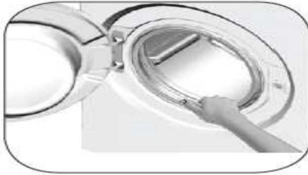
Figure 6.2 Cleaning the bellows
