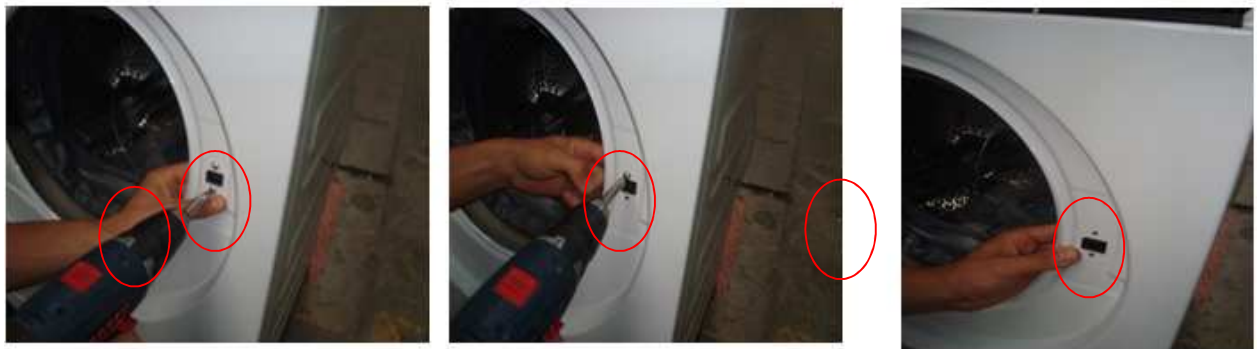
Picture 11.23 Front Wall Disassembly / Assembly
