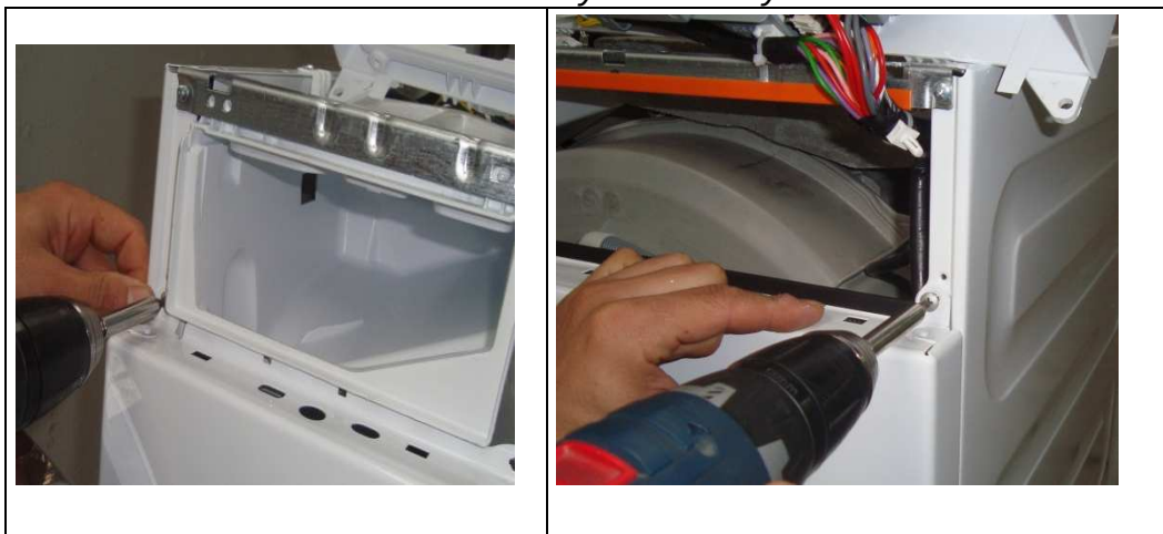
Picture 11.24 Front Wall Disassembly / Assembly
