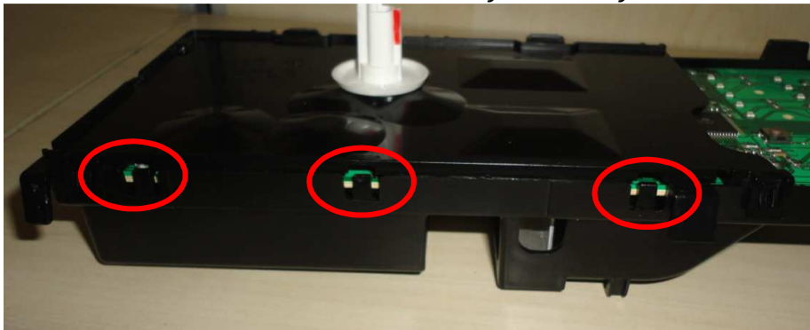
Picture 11.16 Control card Disassembly/Assembly
