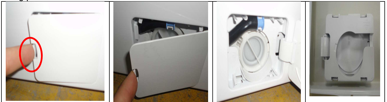
Picture 11.19 Pump cover Disassembly/Assembly
