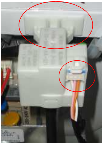
Resim 11.30 Water Level sensör Disassembly/Assembly
