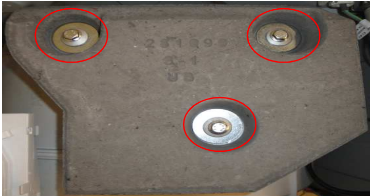
Picture 11.40 Disassembly/assembly of upper counterweight
