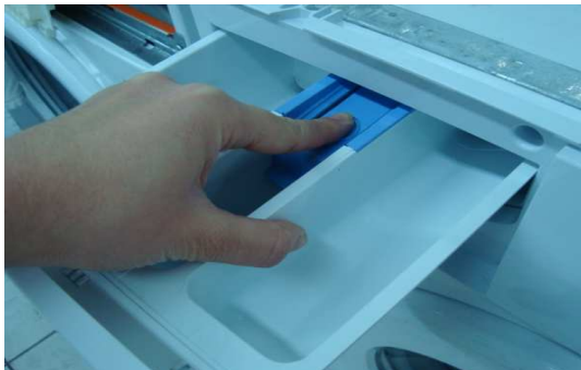
Picture 11.6 Disassembly/Assembly of Detergent Dispenser
