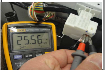
PICTURE E2-5: Water level sensor is being checked
