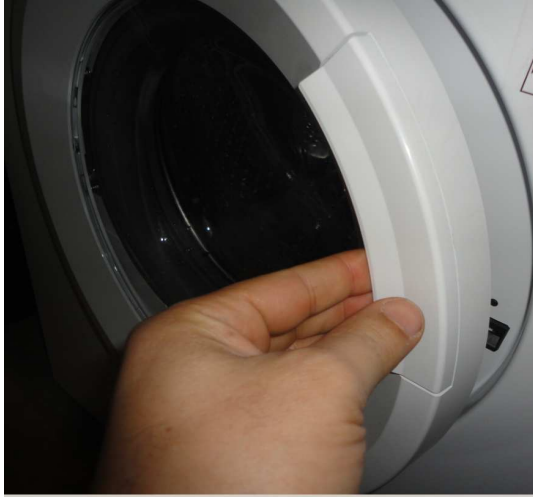
Picture 11.20 Front door disassembly /assembly
