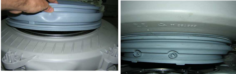
Picture 11.35 Disassembly/Assembly of Drum Bellows
