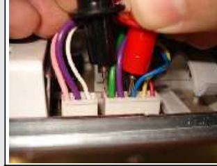
PICTURE E8-3: AC voltage is being measured over valve connectors
