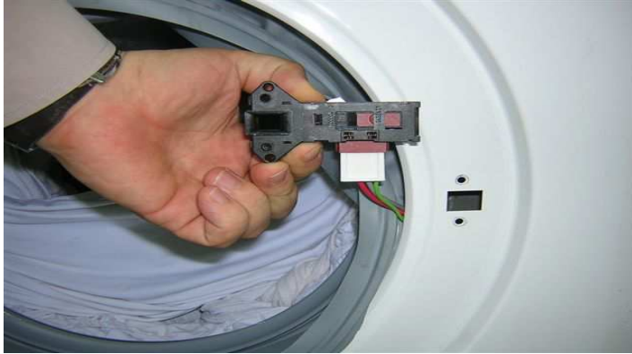
Picture 11.31 Disassembly/assembly of safety switch
