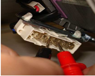
PICTURE E11-5: Motor rotor is being checked over the 8-pin motor
