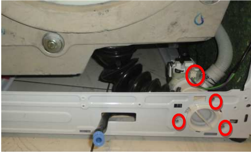
Picture 11.33 Drain pump Attachment/Detachment
