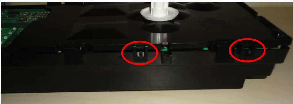
Picture 11.17 Control card Disassembly/Assembly
