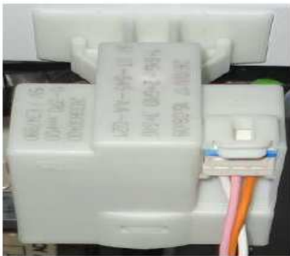
Picture 7.8 Water level sensor
