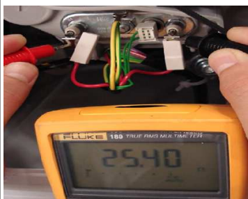
PICTURE E2-4: One of the cables on the heater is removed (left) and heater resistance is measured.
