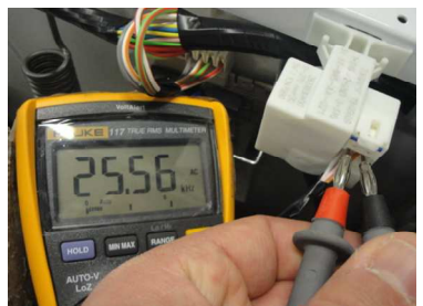
PICTURE E2-5: Water level sensor is being checked
