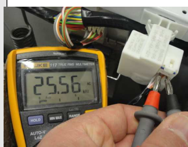
PICTURE E2-5: Water level sensor is being checked
