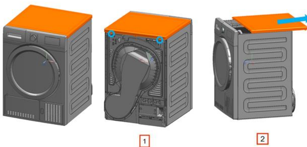
Figure 11.2. Disassembling the top plate
