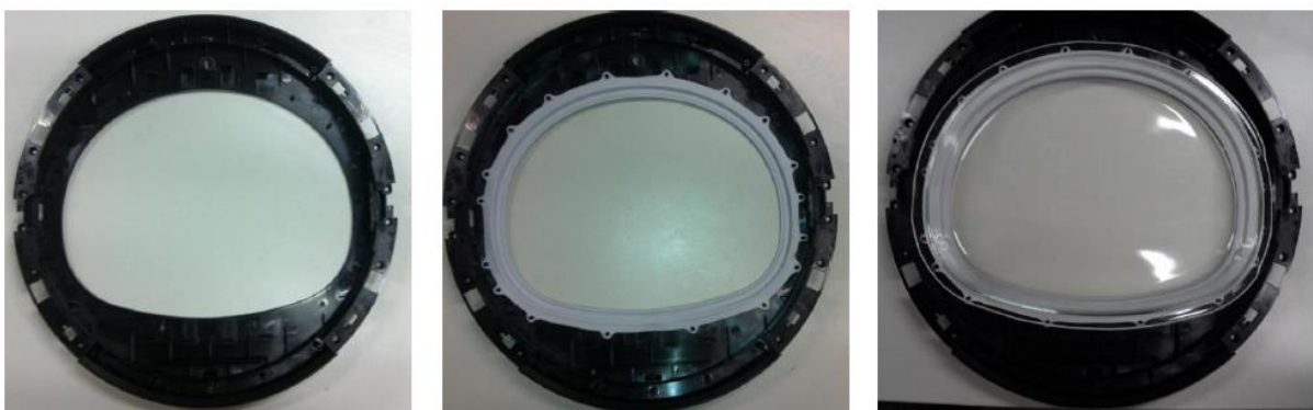
Figure 13.19. Assembling the gasket and glass
