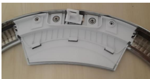
Figure 13.32. The Inner Handle Assembly
